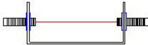
Figure 2: Opposed sensing mode.
