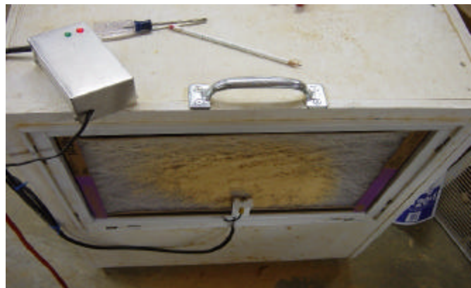
Figure 5: Air-filter with Red LED on with the blockage of the light.
